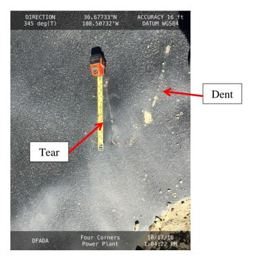
Damage to the geomembrane along the crest of the Cell 1 collection pond. The measuring tape is 12 inches long.
