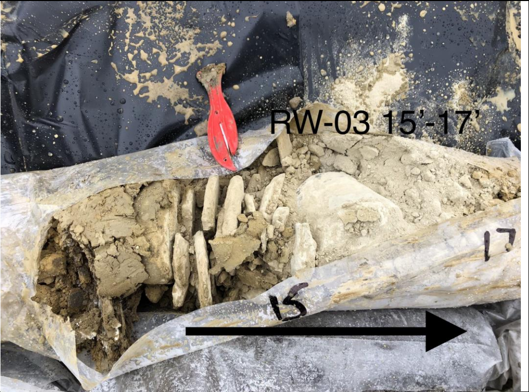
Photograph 40. 15 to 17 ft bgs formation samples from MW-88 (RW-03).
