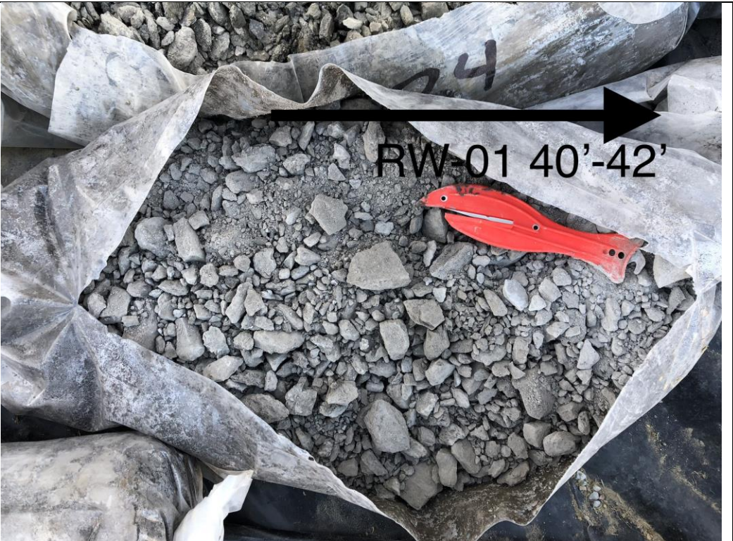
Photograph 20. 40 to 42 ft bgs formation samples from MW-89 (RW-01).
