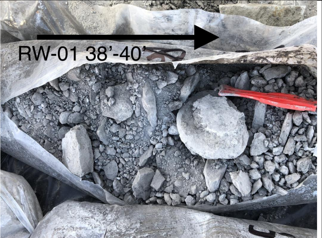
Photograph 19. 38 to 40 ft bgs formation samples from MW-89 (RW-01).
