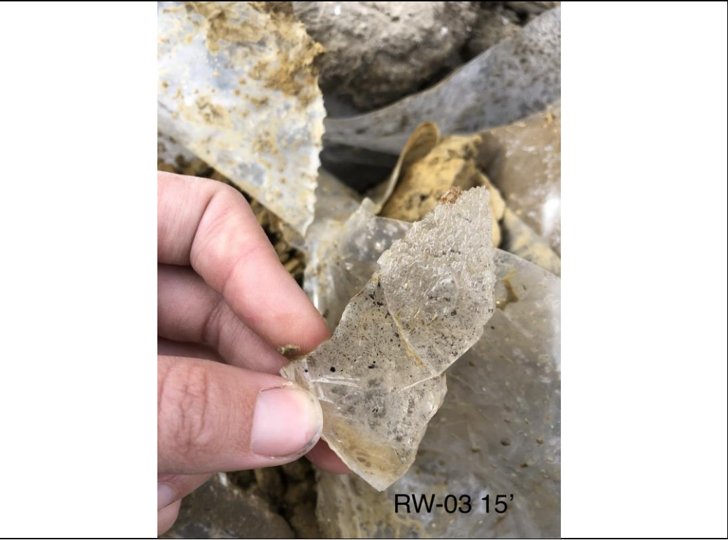
Photograph 38. Gypsum from the 15 ft bgs interval at MW-88 (RW-03).
