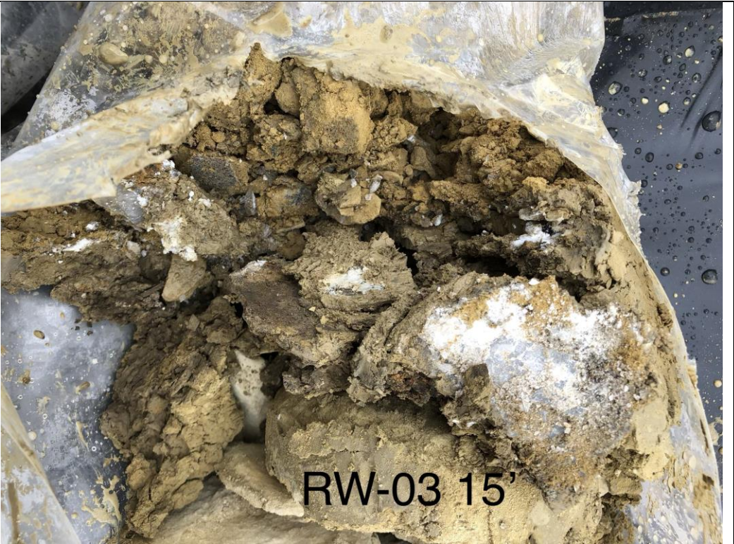
Photograph 39. Weathered shale layer at the 15 ft bgs interval at MW-88 (RW-03).
