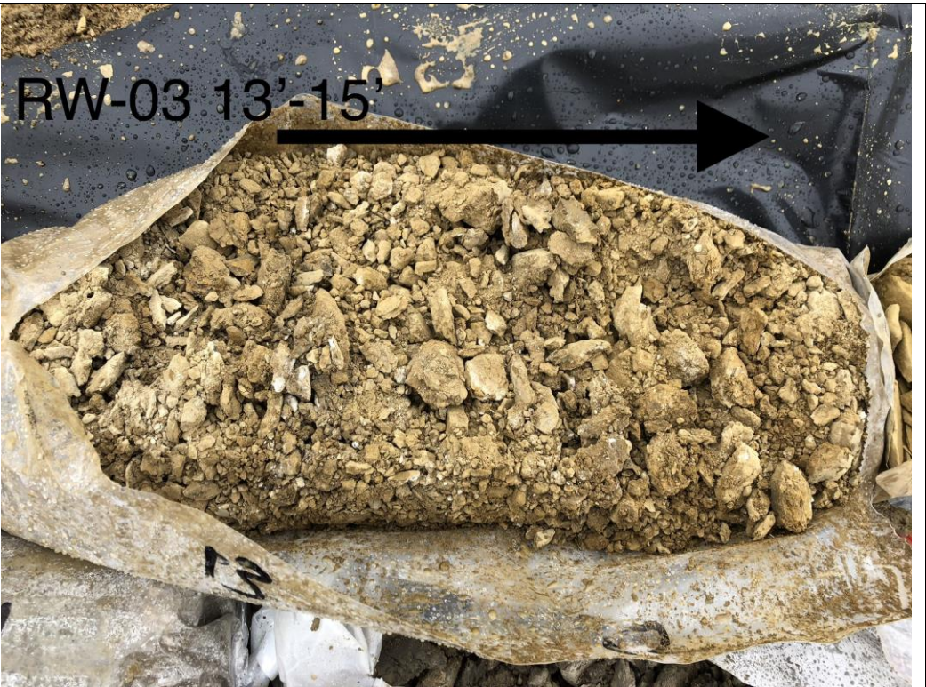
Photograph 37. 13 to 15 ft bgs formation samples from MW-88 (RW-03).
