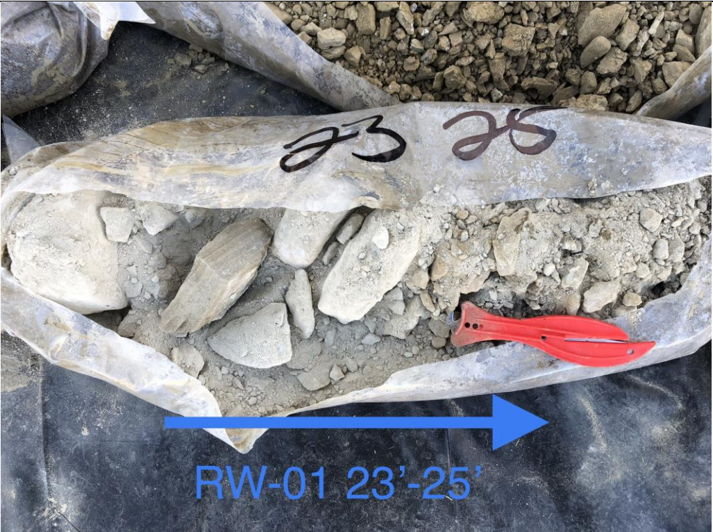
Photograph 11. 23 to 25 ft bgs formation samples from MW-89 (RW-01).
