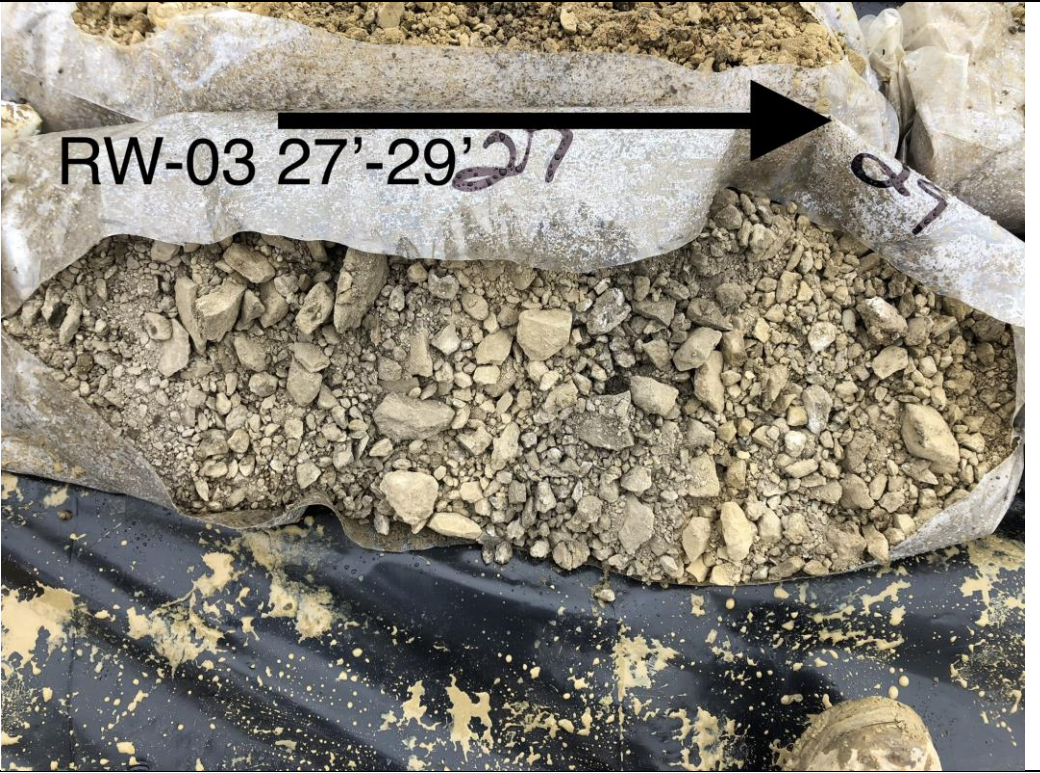
Photograph 46. 27 to 29 ft bgs formation samples from MW-88 (RW-03).
