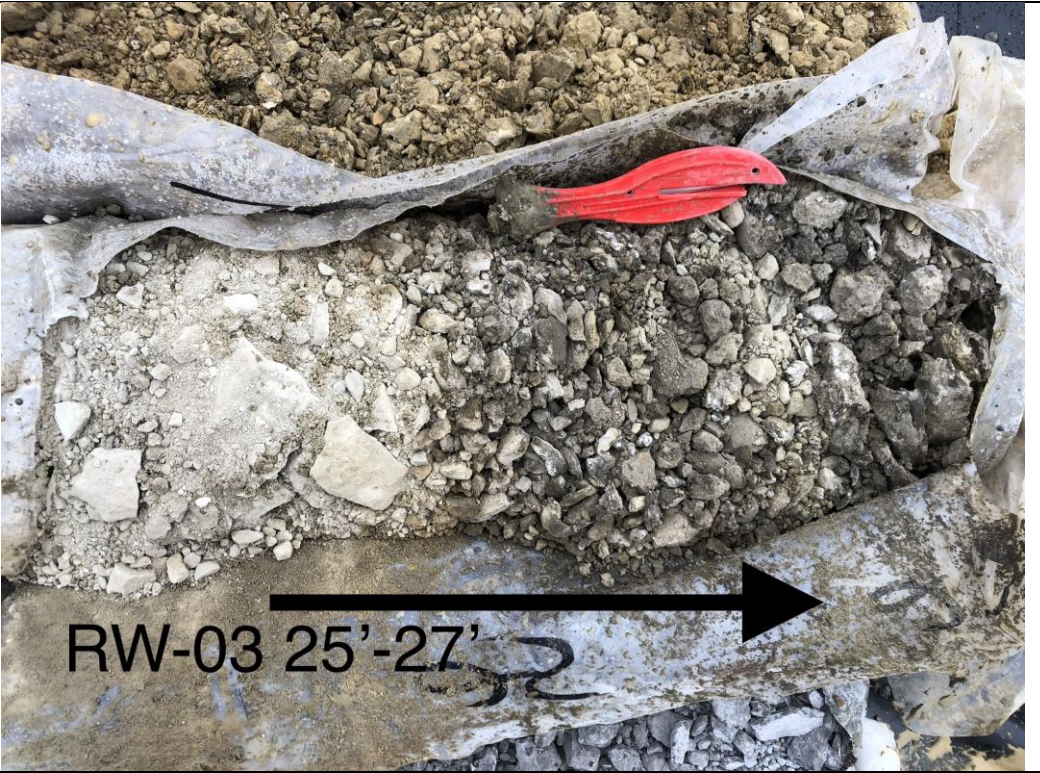
Photograph 45. 25 to 27 ft bgs formation samples from MW-88 (RW-03).
