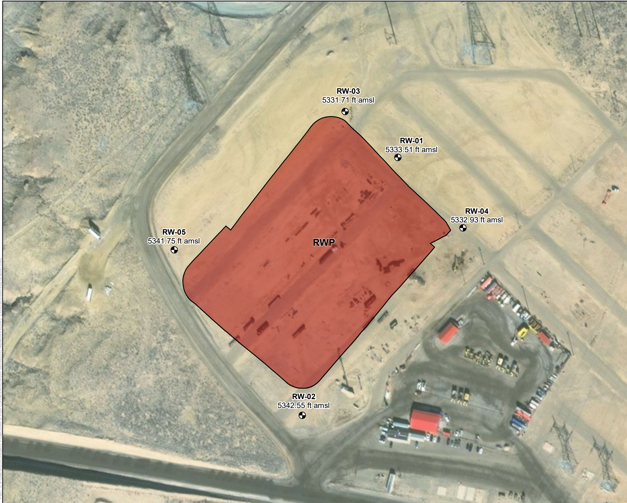
FIGURE 3 Exploratory Boring Location Map Unweathered Lewis Shale Elevations
