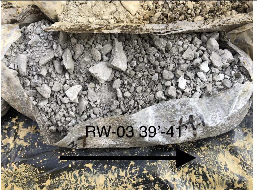
Photograph 52. 39 to 41 ft bgs formation samples from MW-88 (RW-03).
