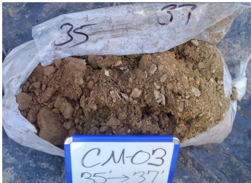
Photo 25: CM-03 soil borings from 35' to 37'.
