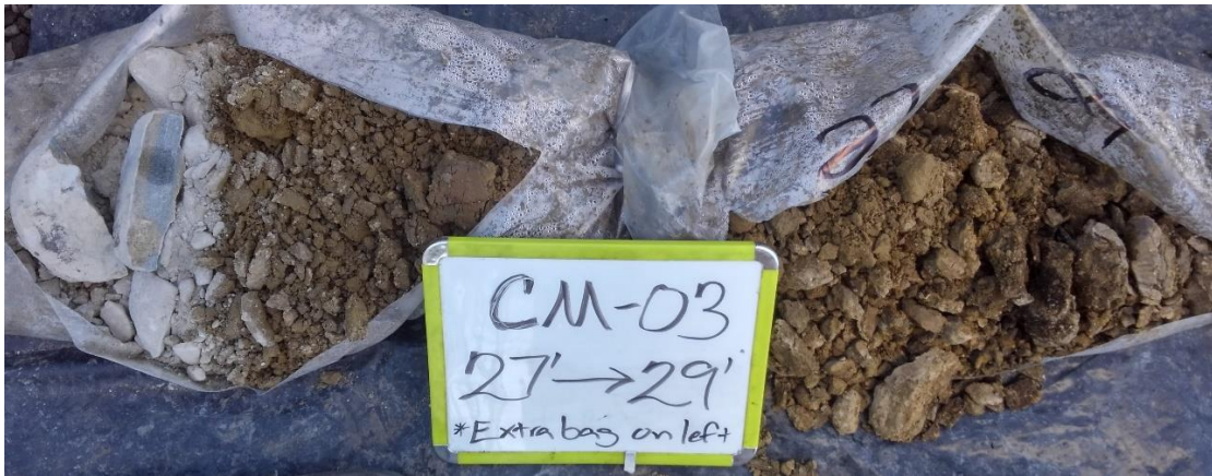
Photo 23: CM-03 soil borings from 27' to 29'.
