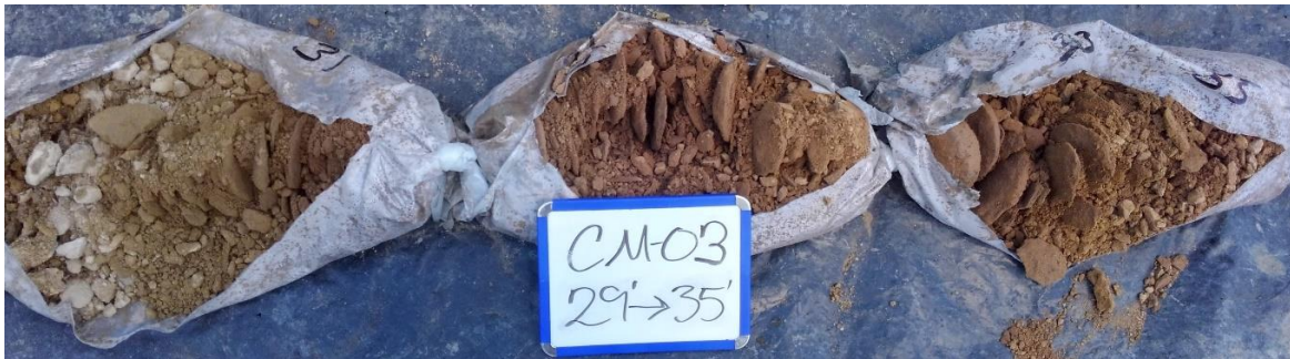
Photo 24: CM-03 soil borings from 29' to 35'.
