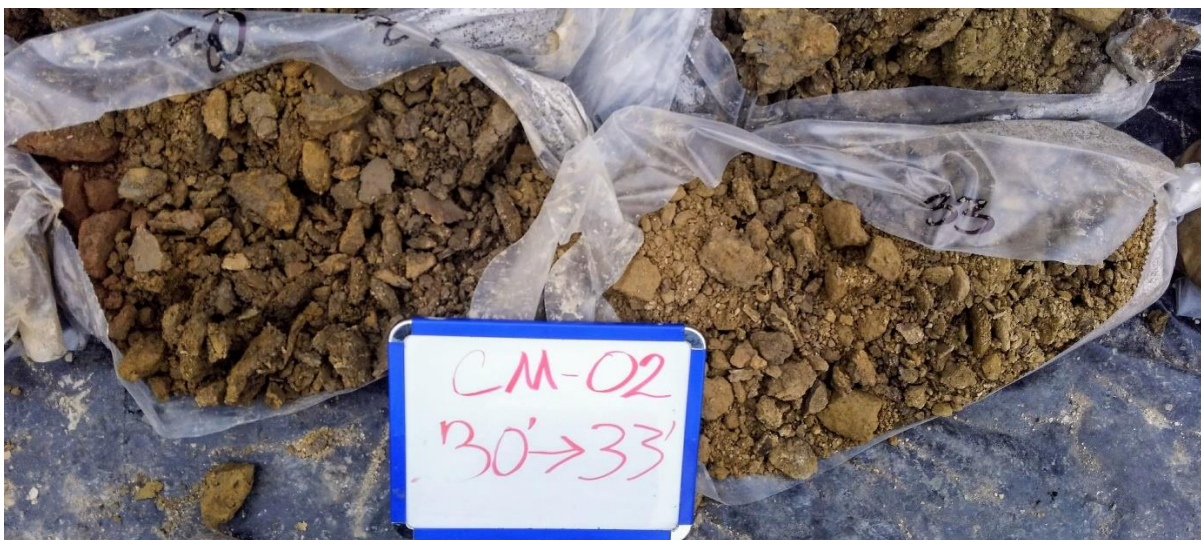
Photo 15: CM-02 soil borings from 30' to 33'.
