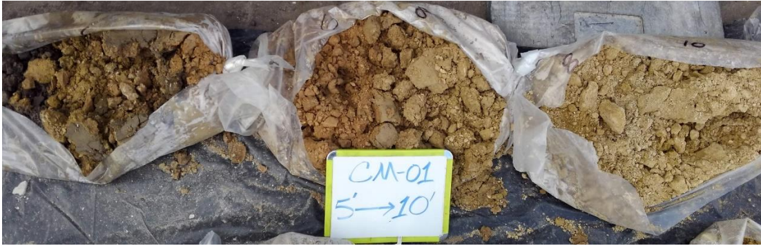
Photo 1: CM-01 soil borings from 5' to 10'.
