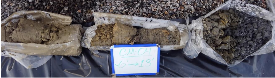
Photo 26: CM-04 soil borings from 6' to 13'.
