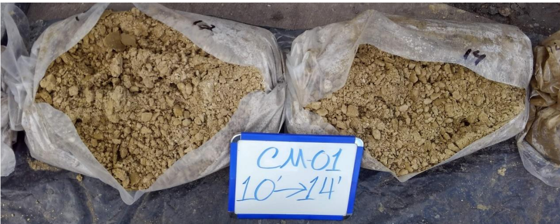
Photo 2: CM-01 soil borings from 10' to 14'.
