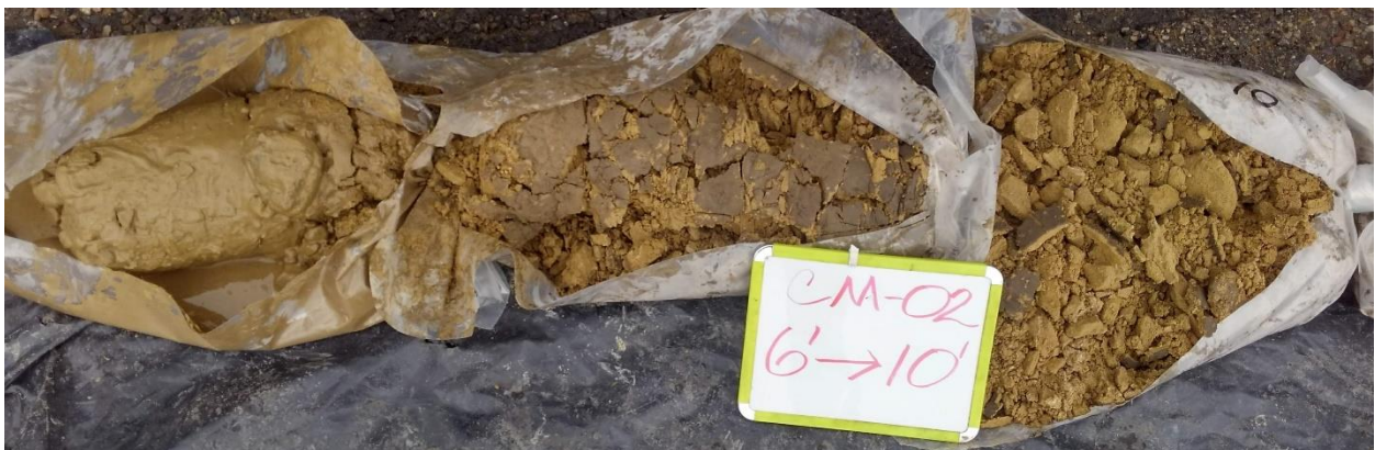
Photo 9: CM-02 soil borings from 6' to 10'.
