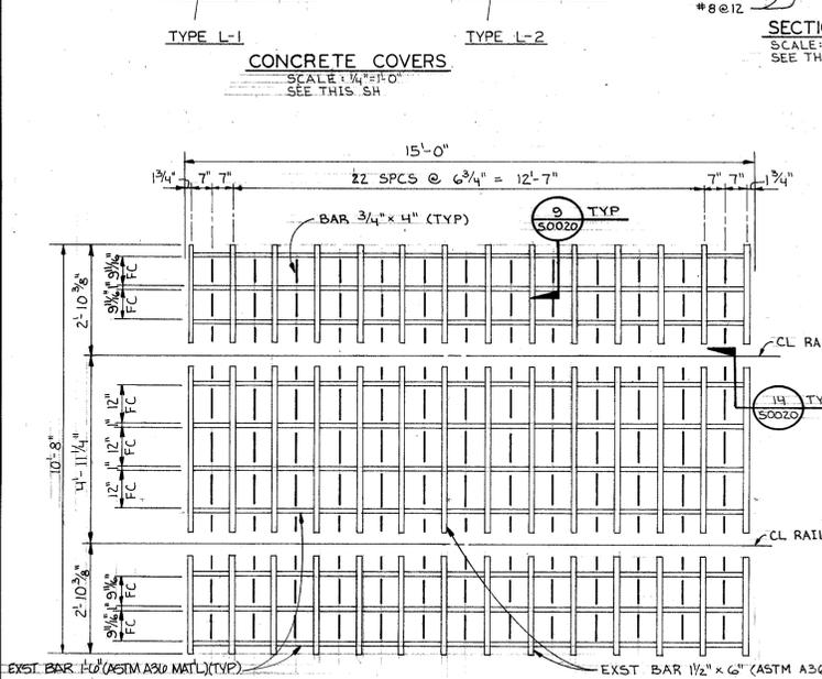
**LIMESTONE UNLOADING HOPPER GRILLAGE MODIFICATION**
