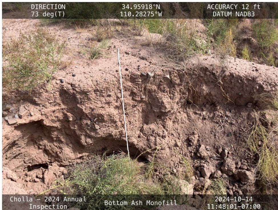
20241014 – IMG_6297 Erosion on the north side of the Stormwater Detention Basin.
