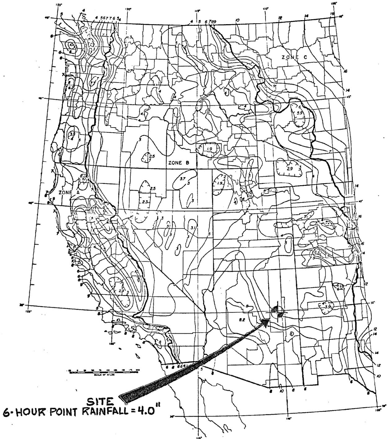
Figure 17. Probable maximum 6-hour point values in inches for general-type storms west of the 105° meridian. 288-D-2756, 288-D-2757.
