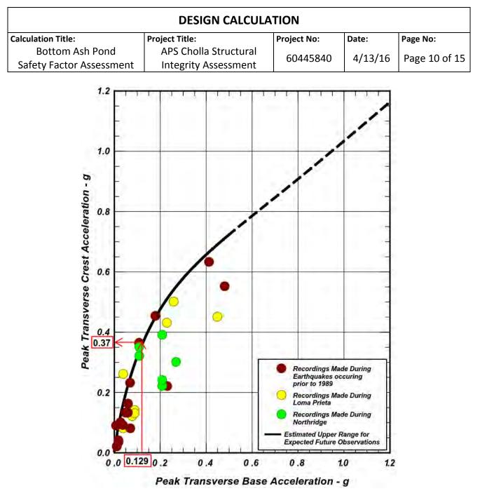
Figure 4. Variations of Peak Transverse Crest Acceleration vs. Peak Transverse Base Acceleration Based on Holzer (1998)
