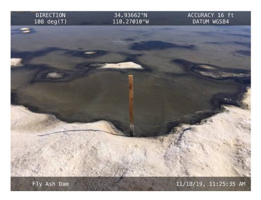
Lathe marking the location where the Fly Ash Pond elevation is measured.
