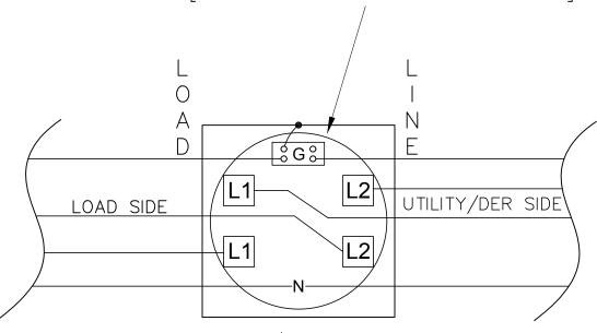
PHOTOVOLTAIC/ENERGY STORAGE PRODUCTION METER [SPECIFY FORM #, MAKE & MODEL #] 240V, 100A, RINGTYPE
