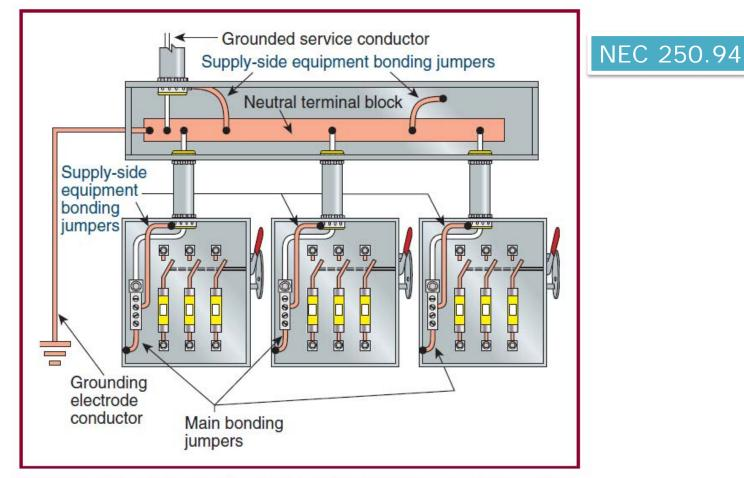
**EXHIBIT 250.34** Grounding and bonding arrangement for a service with three disconnecting means.
