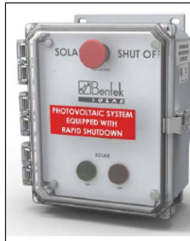
Rapid-shutdown initiator. If loss of ac power does not automatically initiate rapid shutdown, system integrators need to install a manual rapid-shutdown initiation switch—such as Bentek's Rapid Shutdown Controller (left) or MidNite Solar's Bird house (right)—to turn off the array and any battery-backup circuits.
