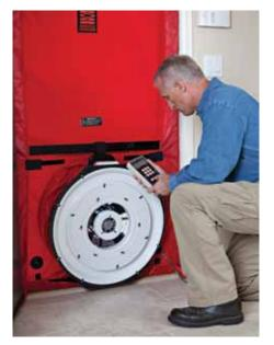
A blower door test is performed to detect leaks in the building envelope.
