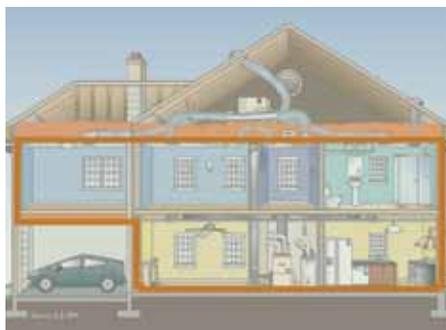
The building “envelope” is indicated by the orange line around the ceiling, walls and floors.
