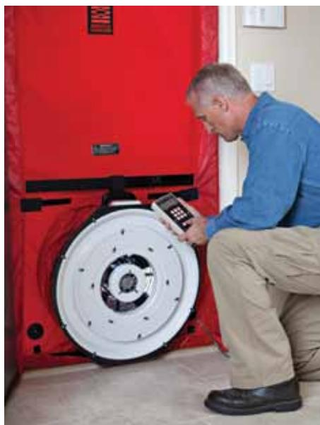
A blower door test is performed to detect leaks in the building envelope.
