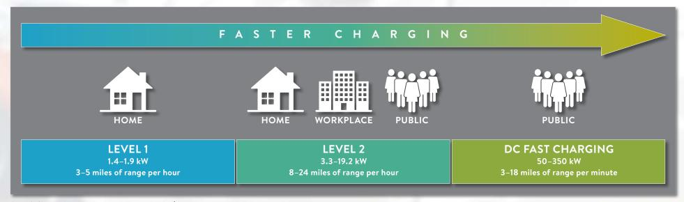
Figure 3. Charging locations, levels, and range replenished<sup>1</sup>
