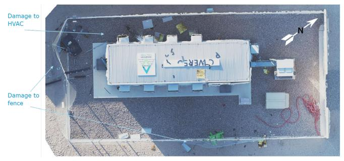
Figure 5 Aerial view of damaged BESS (image credit: Colwell Consulting)
