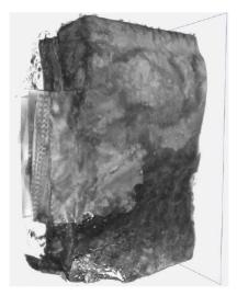
Figure 18 A 3D reconstructed image of the CT-scanned battery cell 7-2 demonstrates the absence of material in the bottom corner of the battery cell (image credit: SEL)
