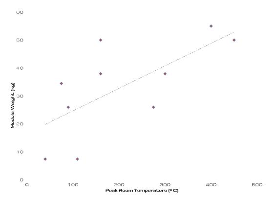
Figure 38 Peak temperatures reached in a thermal runaway testing chamber are directly proportional to the mass of the modules
