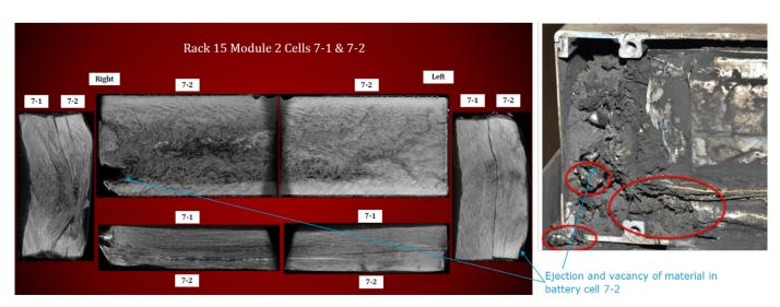
Figure 19 Vacancy of material in battery cell 7-2 during x-ray tomography (left) and evidence of ejected material during the disassembly of Module 2, Rack 15 (right) (images and analysis: SEL)
