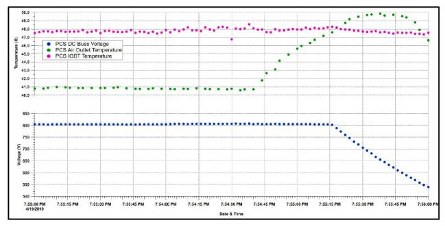
Figure 15 Air temperatures increased as voltage in Rack 15 declined (image and analysis: SEL)
