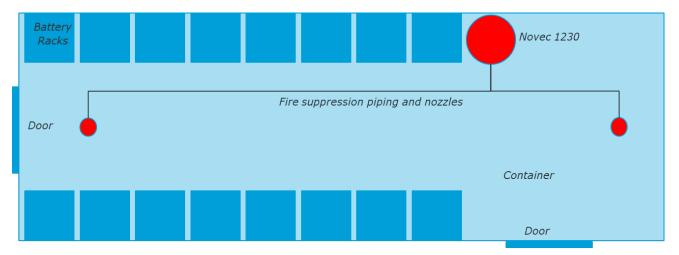
Figure 4 A simplified illustration of a typical fire suppression system within an energy storage container similar to McMicken
