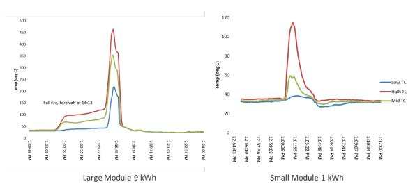
Figure 32 Comparison of temperature during a fire test, large modules vs. small modules
