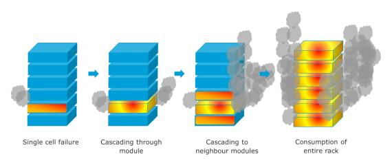
Figure 25 A single cell failure propagated through Module 2, then consumed the whole rack, releasing a large plume of explosive gases. This process could have occurred without visible flame, which would explain why the gases were not burned as they were emitted.
