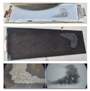
Figure 20 Deposits and dendritic growth observed on other McMicken battery cells during the investigation (image credit: SEL)
