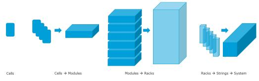
Figure 2 Generalized system architecture
