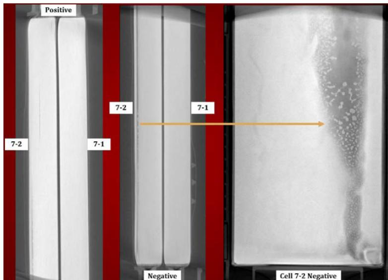
**Figure 21 Deposits and dendritic growth observed in other McMicken battery cells outside of Rack 15 (Rack 24, Module 6, Cells 7-1 and 7-2) (image credit: SEL)**
