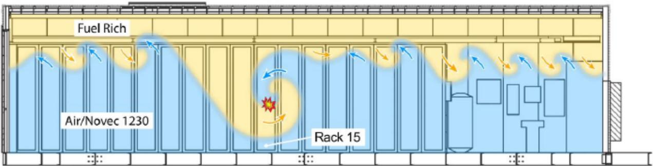
**Figure 27 Colwell’s simplified illustration of flammable gases near the top of the container rolling back as a reaction to the door opening, putting them in contact with residual heat or spark at Rack 15 (image credit: Colwell)**
