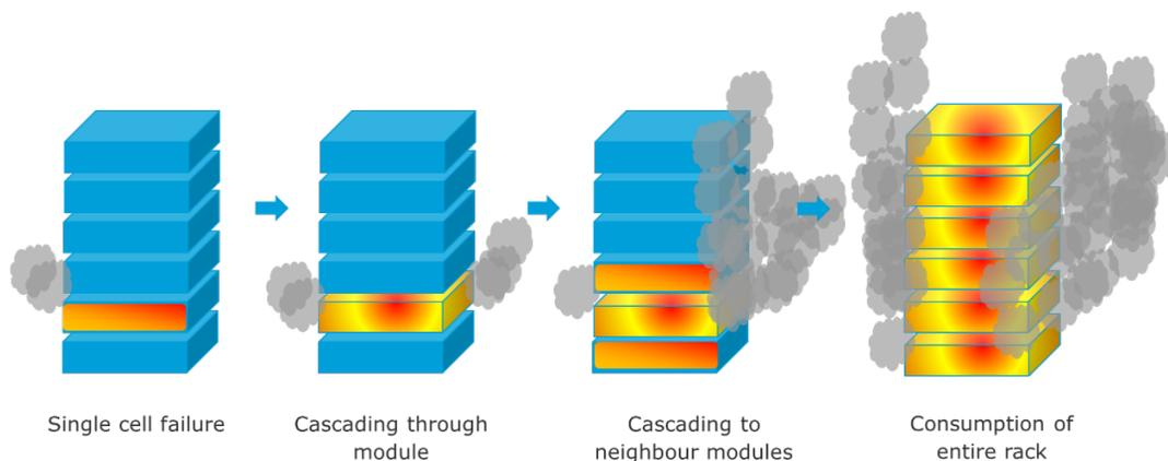
**Figure 25 A single cell failure propagated through Module 2, then consumed the whole rack, releasing a large plume of explosive gases. This process could have occurred without visible flame, which would explain why the gases were not burned as they were emitted.**
