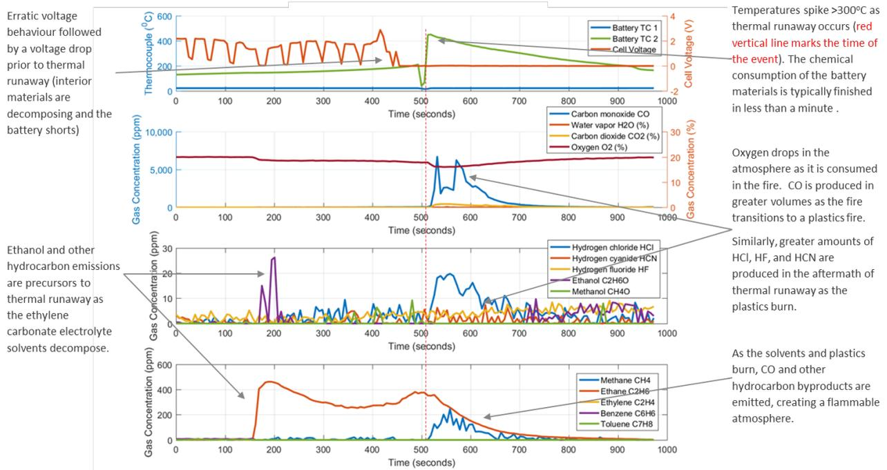
**Figure 12 A typical pattern of a Li-ion battery cell thermal runaway event in air with observed temperature behavior and gases**
