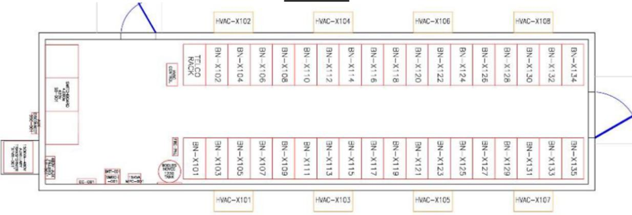
**Figure 17** Rack numbering layout inside the energy storage container
