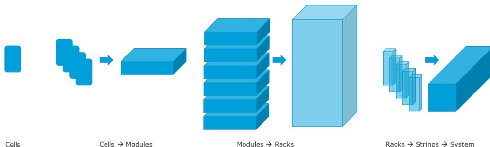
**Figure 2 Generalized system architecture**
