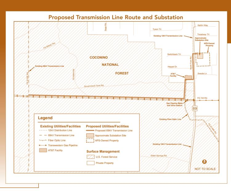
From U.S. 89, the proposed route would extend west along the south side of the existing AT&T facility. The line would turn south again, following the AT&T fiber optic corridor until reaching a natural gas pipeline corridor which currently contains two natural gas pipelines. Within this corridor, the line would extend west, parallel to the northernmost gas pipeline before connecting with the existing APS Tuba City-Flagstaff 69-kV transmission line approximately 1.5 miles west of U.S. 89.
