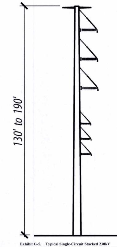
ibit G-5. Typical Single-Circuit Stacked 230kV Monopole with Single-circuit Stacked 69kV Underbuild Transmission Structure
