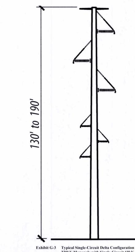
hibit G-3 Typical Single-Circuit Delta Configuration 230kV Monopole with Single-Circuit 69kV Underbuild Transmission Structure
