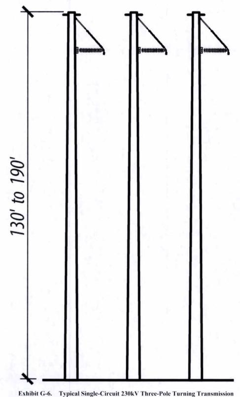
Typical Single-Circuit 230kV Three-Pole Turning Transmission Structure
