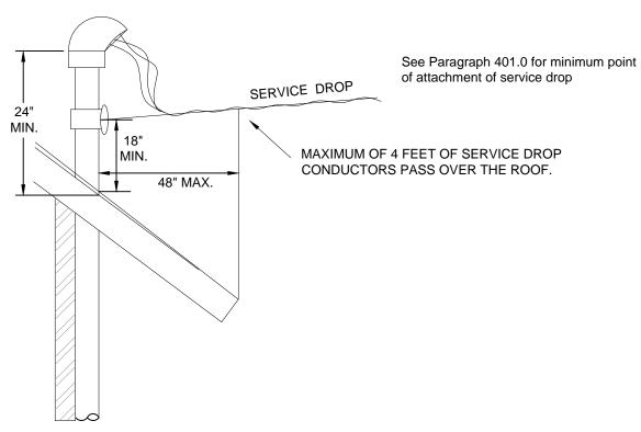
Service entrances shall not be located within a roofed-over area necessitating APS personnel to walk on, or place a ladder on roof to make attachment to riser conduit or support, and to connect Customer's service.
