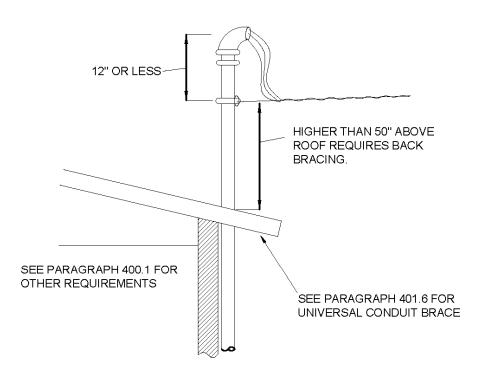
**BACK BRACING:** Risers that require back bracing shall be braced against the pull of the service drop conductors. Back bracing shall consist of two steel members installed at approximately a 90 degree spread. Minimum size braces shall be 3/4" rigid galvanized steel pipe or 1 1/4" x 1 1/4" x 1/8" steel angle.
