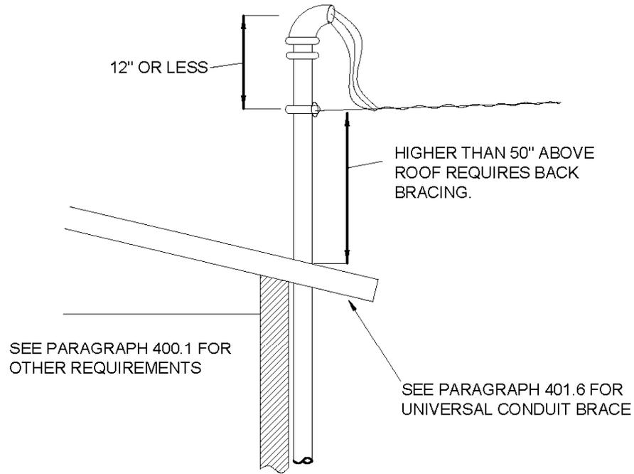
**BACK BRACING:** Risers that require back bracing shall be braced against the pull of the service drop conductors. Back bracing shall consist of two steel members installed at approximately a 90 degree spread. Minimum size braces shall be 3/4" rigid galvanized steel pipe or 1 1/4" x 1 1/4" x 1/8" steel angle.
