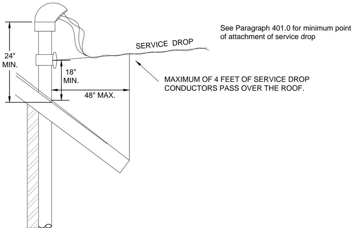
Service entrances shall not be located within a roofed-over area necessitating APS personnel to walk on, or place a ladder on roof to make attachment to riser conduit or support, and to connect Customer's service.
