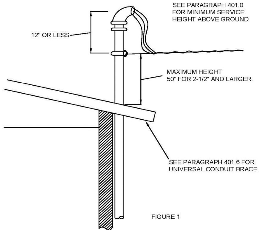
Where the service conduit riser is used as a mast for supporting the service drop, the point of attachment shall not be higher than 50" above the roof unless substantially braced (not guyed) on the roof to provide sufficient strength to support the strain of the service conductors, and to permit a man to work safely from a ladder bearing against the conduit. (See Paragraph 401.5 for alternative to bracing for residential.)
