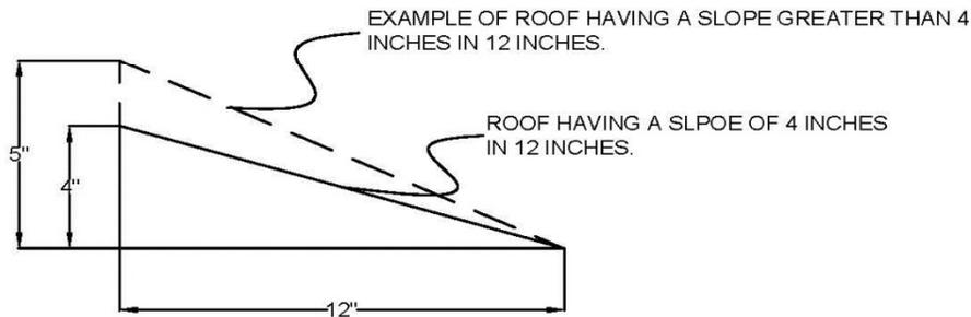
The intent of this exception is that where the roof has a slope 4 in. in 12 in. or greater it is considered difficult to walk upon and the height of conductors could then be less than 8 ft. from the highest point over which they pass but in no case less than 3 ft. except as permitted in Exception 2.
