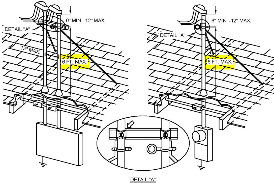
NEED BACK BRACE IF 2" RISER IS HIGHER THAN 30" ABOVE PARAPET WALL BRACE
