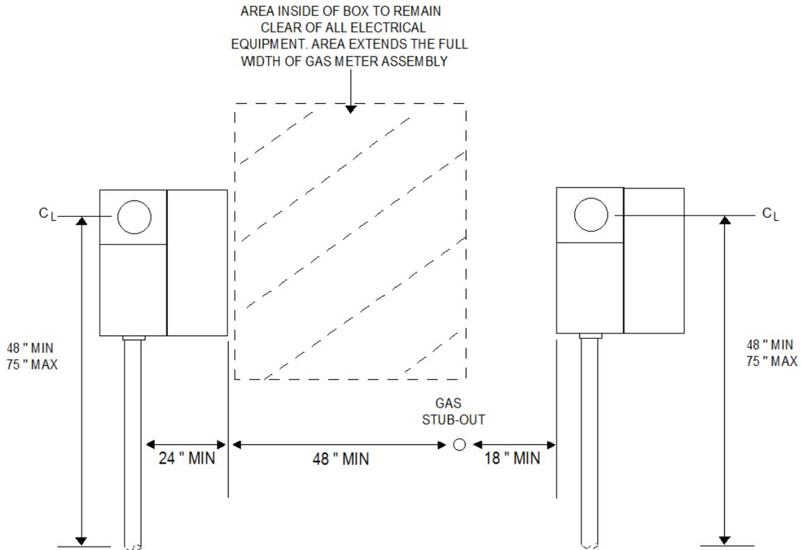
**301.15-2 ESTABLISHING GAS CLEARANCES DURING CONSTRUCTION (FIGURE 2)**
