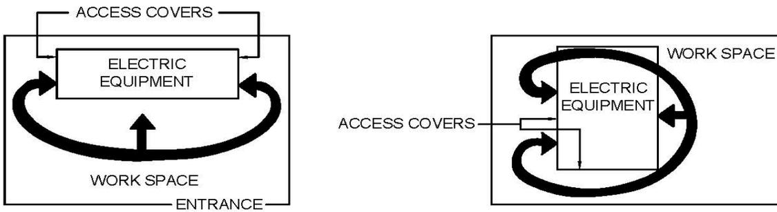
AT LEAST ONE ENTRANCE IS REQUIRED TO PROVIDE ACCESS TO THE WORKING SPACE AROUND ELECTRIC EQUIPMENT. THE INSTALLATION SHOWN IN THE SKETCH ON THE RIGHT WOULD NOT BE ACCEPTABLE IF THE ELECTRIC EQUIPMENT WAS A SWITCHBOARD OR PANELBOARD OVER 6' WIDE AND RATED 1200A OR MORE.
