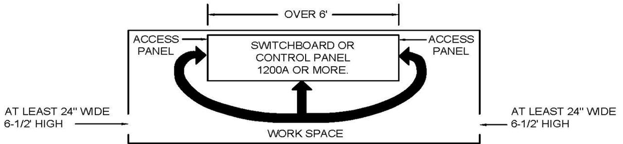
FOR SWITCHBOARDS AND CONTROL PANELS RATED 1200A OR MORE AND OVER 6' WIDE, THERE SHALL BE ONE ENTRANCE NOT LESS THAN 24" WIDE AND 6-1/2' HIGH AT EACH END.
