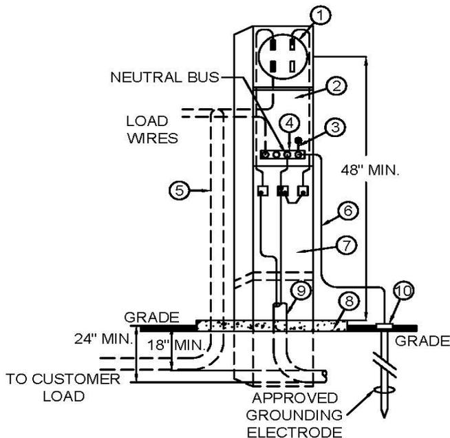
THIS IS A LIST OF MATERIAL FOR A NORMAL METER PEDESTAL INSTALLATION. IT IS NOT INTENDED TO BE ALL INCLUSIVE BUT GIVES THE MORE COMMON REQUIREMENTS. ALL EQUIPMENT SHALL COMPLY WITH EUSERC REQUIREMENTS (SEE SECTION 1100, DWG. 307) AND SECTION 500, PARAGRAPH 506.6-1, 2.
