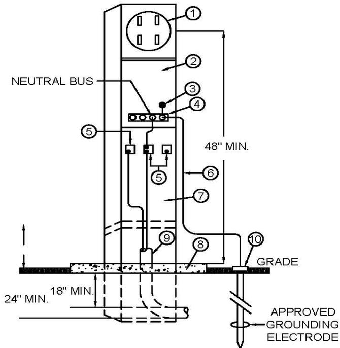
THIS IS A LIST OF MATERIAL FOR A NORMAL METER PEDESTAL INSTALLATION. IT IS NOT INTENDED TO BE ALL INCLUSIVE BUT GIVES THE MORE COMMON REQUIREMENTS. ALL EQUIPMENT SHALL COMPLY WITH EUSERC REQUIREMENTS (SEE SECTION 1100, DWG. 307) AND SECTION 500, PARAGRAPH 506.6-1, 2.
