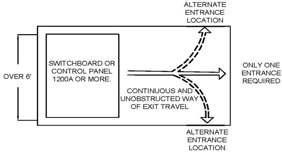
EXCEPTION #1: WHERE THE EQUIPMENT LOCATION PERMITS A CONTINUOUS AND UNOBSTRUCTED WAY OF EXIT TRAVEL.
