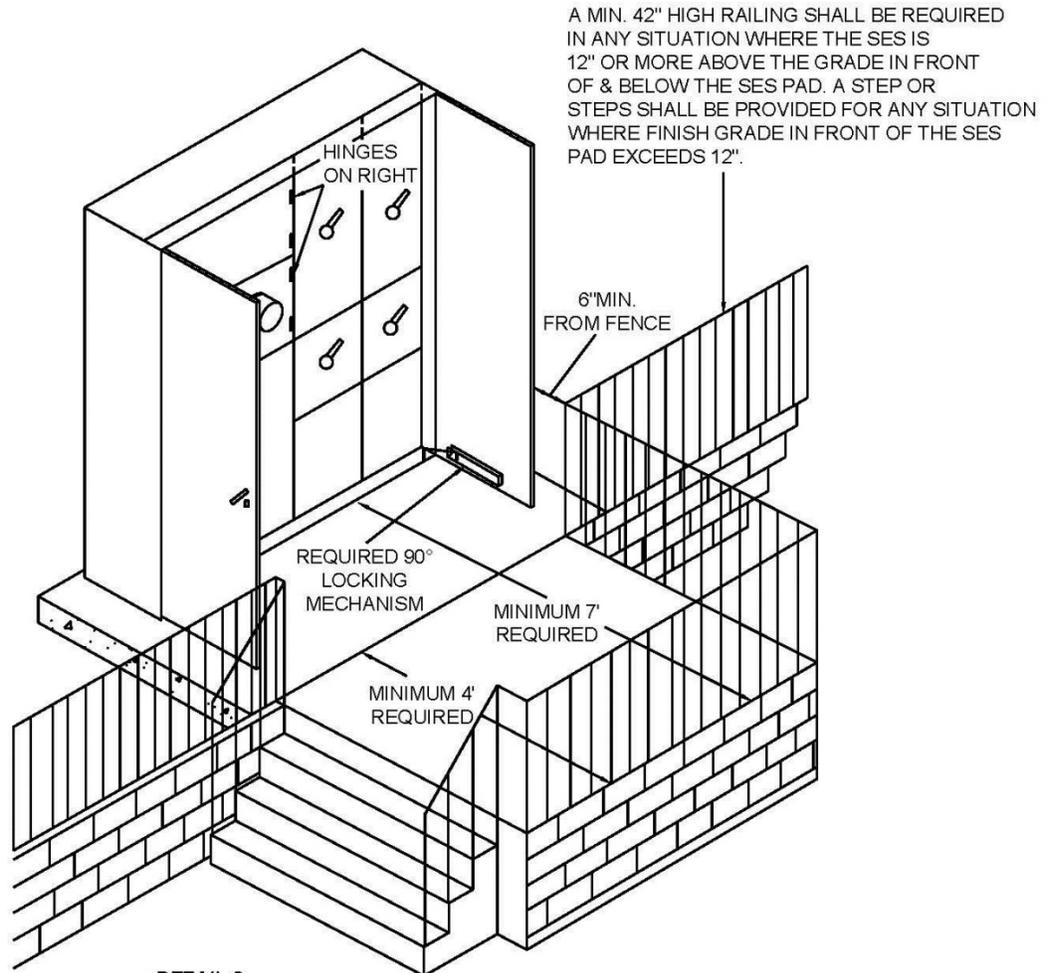
A MIN. 42" HIGH RAILING SHALL BE REQUIRED IN ANY SITUATION WHERE THE SES IS 12" OR MORE ABOVE THE GRADE IN FRONT OF & BELOW THE SES PAD. A STEP OR STEPS SHALL BE PROVIDED FOR ANY SITUATION WHERE FINISH GRADE IN FRONT OF THE SES PAD EXCEEDS 12".
