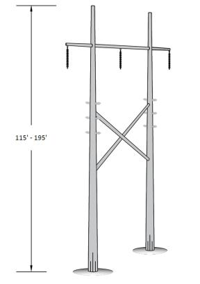
**Exhibit G3** Single-Circuit 230kV H-Frame with Double-Circuit 69kV Underbuild Capable
