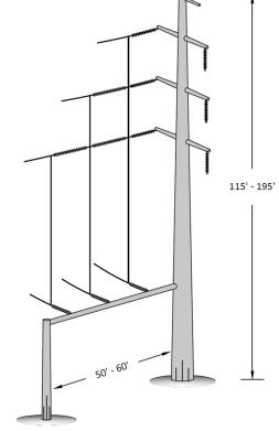
**Exhibit G4** Single-Circuit 230kV Cut-In / Single-Circuit 230kV Tangent
